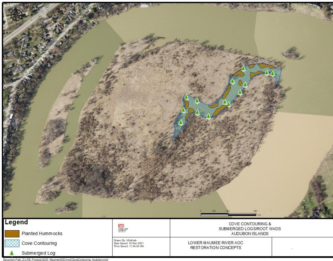
Figure 43: Cove contouring with planted hummocks and submerged trees/root wads.
