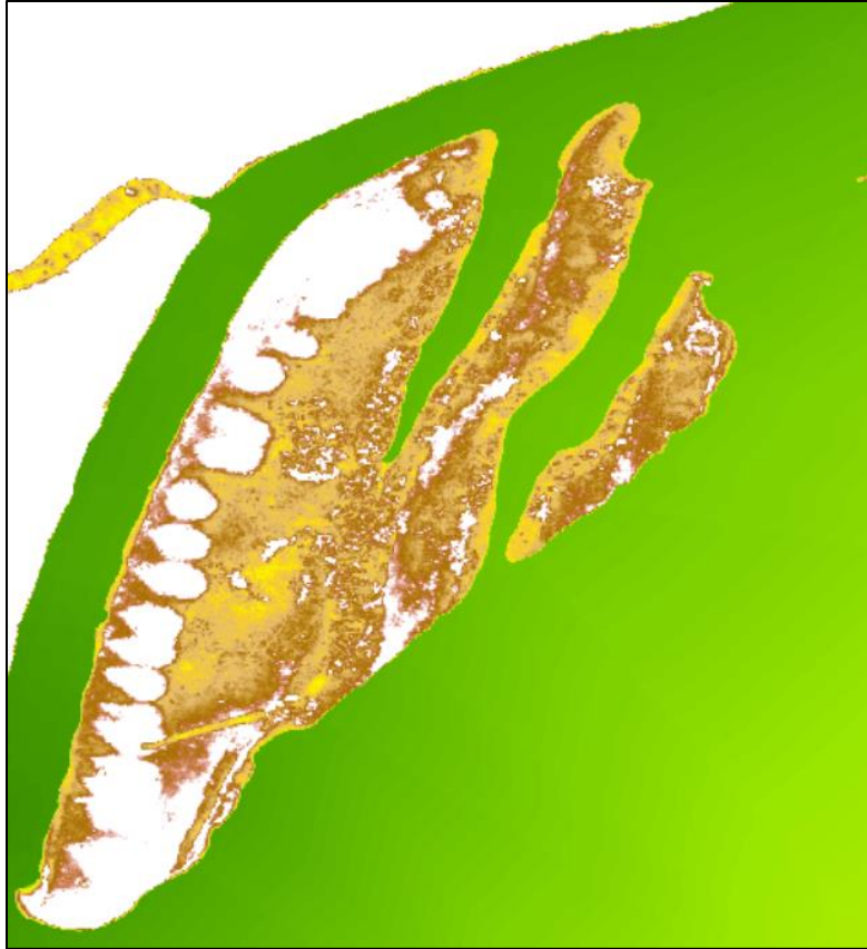
Figure 25. Delaware/Horseshoe Island: Areas above Maximum Monthly Average Lake Erie Level (White) and Areas below (Colors).
