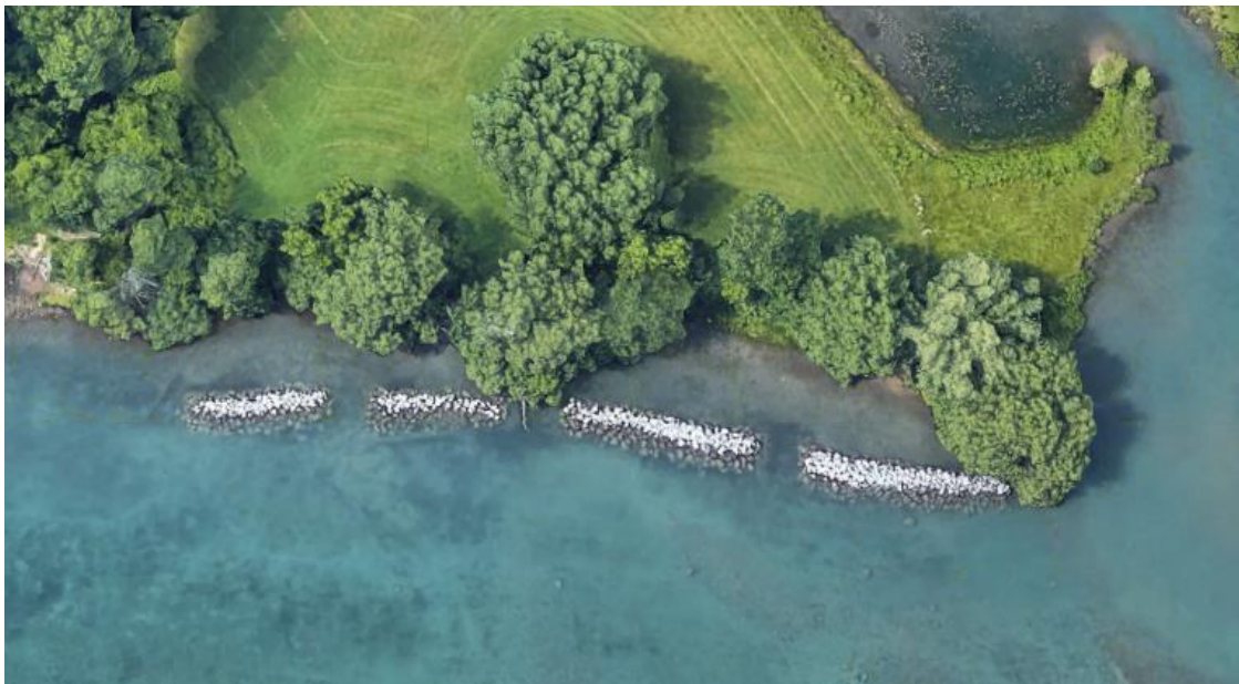
Figure 34: Detached rock reefs along the shoreline of Beaver Island, Grand Island, NY. Source, Google Earth 2021.
